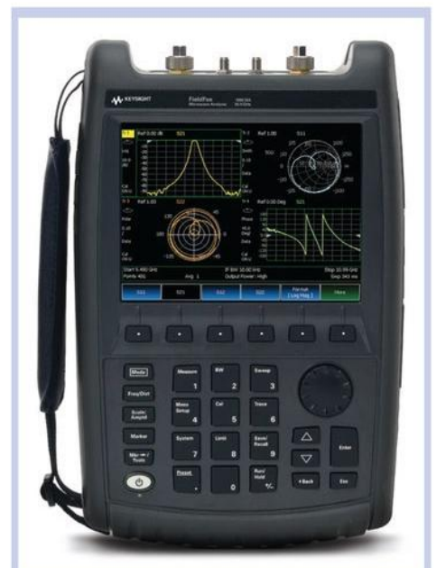
■ FIGURE 1. This portable spectrum analyzer is the best way to find EMI of the RF wireless sort. Courtesy Keysight Technologies.
